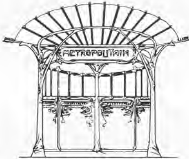
50 Guimard, iron and glass Métro entrance, Paris, 1899–1904. Side and front elevations.
