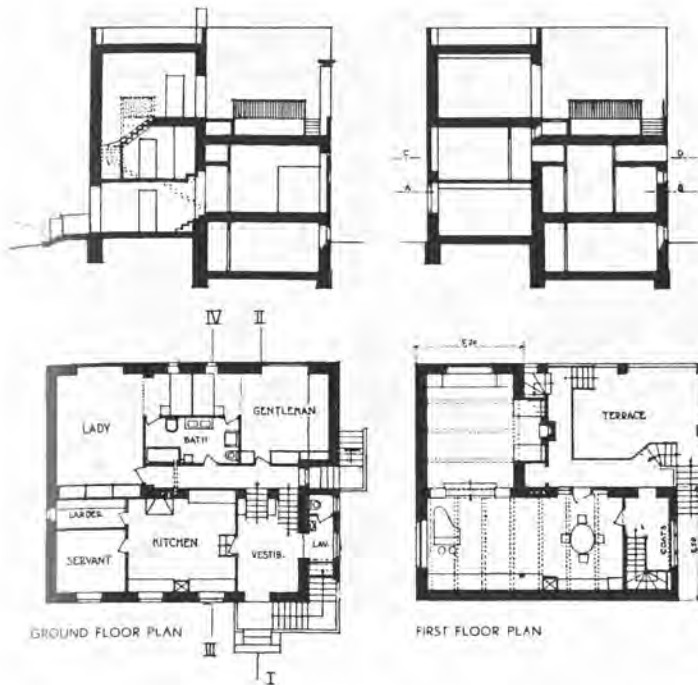
74, 75 Loos, villa project for the Venice Lido, 1923. Left , transverse sections (through I-II and III-IV), and plans of ground and first floor: below , model.
